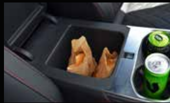
PIE WARMER/DRINKS COOLER: CENTRE CONSOLE HOT + COOL BOX (RUNS OFF AC SYSTEM)
